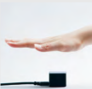
Sensor transmits infrared radiation to the hand, venous blood absorbs infrared rays
